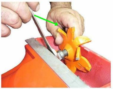
While holding the cutter with one hand, turn the shaft with the spanner following the direction of arrow as shown on picture. Repeat this movement twice or three times until shaft thread has entered the cutter. Continue screwing on the cutter with the hand as usual.
