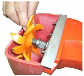
To screw on RZ-150 cutter, place it opposite to the shaft and press softly against thread.
